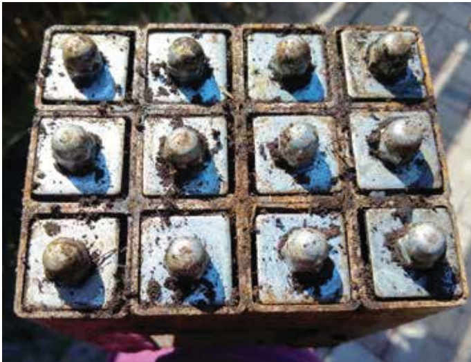
Underside of the soil blocker with square washers and cap nuts clearly visible
